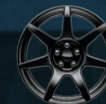
19" x 11.0" front 19" x 11.5" rear EBONY BLACK-PAINTED CARBON FIBER Included with R Package
